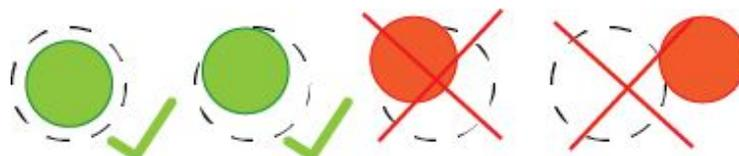
*Pict. 6 - The probe must be inside the circles (1st and 9th calibration point) to successfully level the bed.*
